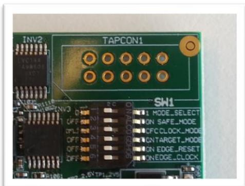
This DIP Switch is used to configure transparent and non-transparent modes, set and select the clock source.
