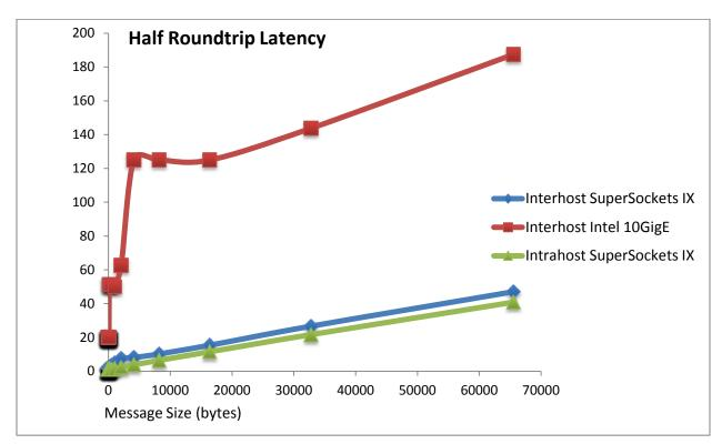
As is shown in the previous chart *SuperSockets™* accelerates both inter-host transfers between separate servers, and intra-host transfers within a host server.
