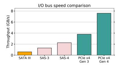
Figure 1: Throughput of PCIe compared to other traditional I/O buses. Consumer NVMe drives today are able to saturate a PCIe x4 bus for sequential reads.
