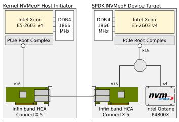
(c) Accessing a remote drive over IB using the kernel NVMeoF using RDMA driver.
