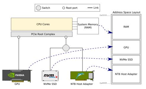
Figure 4: The system enumerates the PCIe device tree and maps device memory regions it on the same address space as system memory. Devices that are capable of DMA can access system memory as well as other devices on the PCIe fabric.
