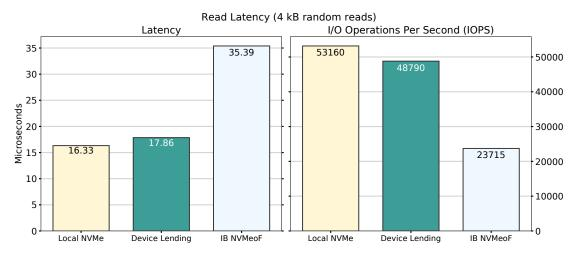
Figure 9: Results of our NVMeoF access latency benchmark using the Linux kernel driver stack. The benchmarking program executed 327,680 reads of 4 kB each, using a random pattern.
