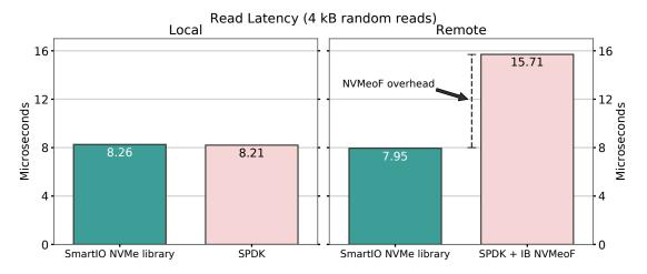
Figure 10: Results of our NVMeoF access latency comparison between SPDK and our SmartIO NVMe library. The FIO benchmarking program executed 327,680 reads of 4 kB each, using a random pattern. Note the overhead added by the NVMeoF protocol.
