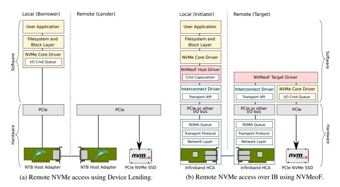
Figure 7: Device Lending makes the remote NVMe drive appear local, eliminating the need for forwarding I/O commands and RDMA transactions to the remote system. Instead, the local NVMe driver can access the drive directly over PCIe.
