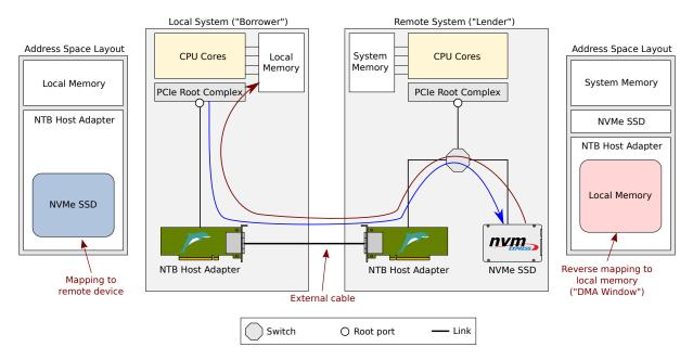
Figure 5: By mapping a remote device's memory over an NTB, a local CPU may read from and write to it. Likewise, local system memory can be mapped for the remote device, allowing it to access local memory using DMA.
