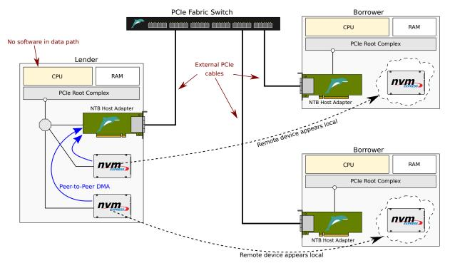
Figure 6: The Device Lending mechanism uses memory mappings to make remote devices appear as if they are installed locally. Since devices can be borrowed and returned dynamically, Device Lending is a highly flexible approach to composing the I/O infrastructure in PCIe clusters.
