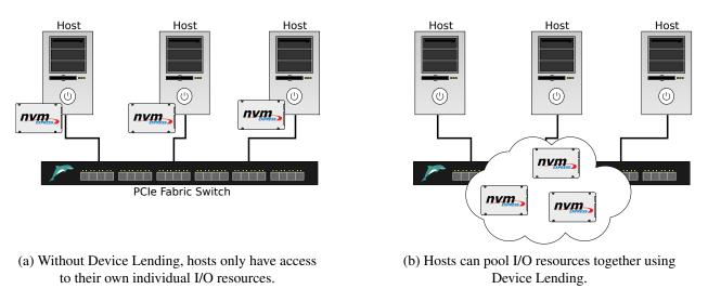
Figure 3: With Device Lending, devices become decoupled from the physical hosts they reside in. We can imagine this as connected hosts in a cluster contributing to a shared pool of I/O resources.
